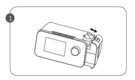
Remove the humidifier chamber.
