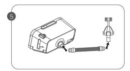
Connect one side of the tube to the air outlet and mask at the other end.
