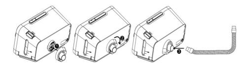
**Note:** If you are using a standard tube (not shown) instead of a heated tube, simply slide the tubing over the air outlet port on the therapy device.
