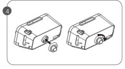
Lock the outlet onto back of device by turning outlet clockwise.
