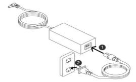
3. Plug the power supply cord's connector into the power inlet on the side of the device.
